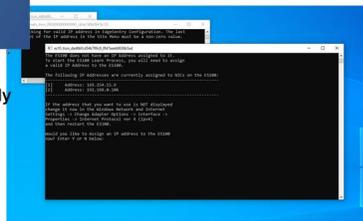
**If the networked system is NOT complete** - leave the system in this state (power it down if you like) and finish the remaining work on the network prior to putting the ES100 into "Learn" mode.
