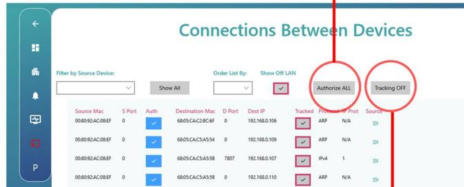
Turn tracking ON if you want to have the device connection recorded in the Tracking Report. Try to use this selectively as the Tracking Report can get very long quickly! The system will automatically stop tracking devices once there are more than 5000 tracked devices listed.
